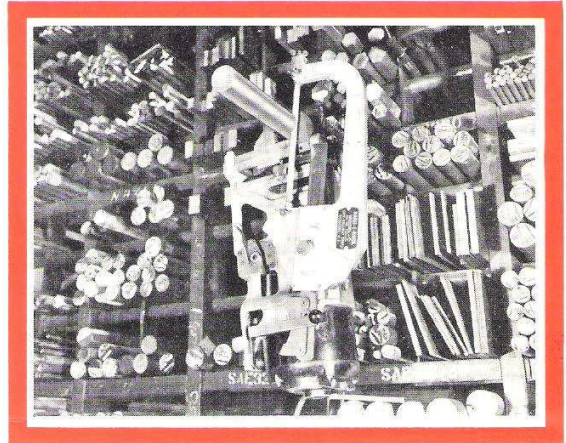
Here the Hand-I-Hack is hanging on its work while making a cut in the stockroom.
