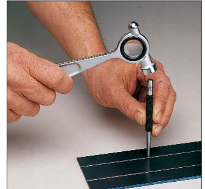
Locating hole center on a workpiece with Starrett No. 816 Prick Punch and No. 815 Toolmakers' Hammer.
